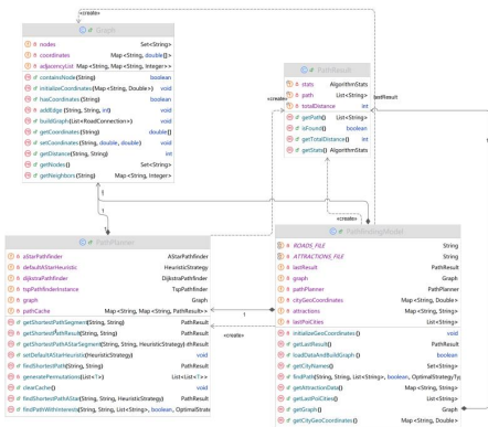
Figure.3 Class Diagram of the Model Components
