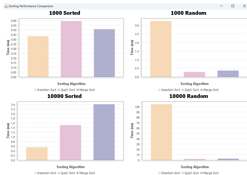
Figure.13 Execution time comparison of three sorting algorithms
